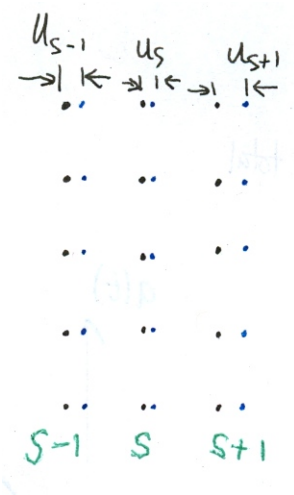
Figure 20: The vibrations of 3 lines of planes of lattice points. Notice that each point (on a line) moves from its equilibrium by a different amount (between lines), but the same amount on a line.
